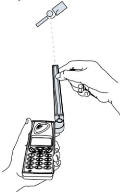
If you are closer to the edge of the satellite's coverage area than the centre, angle the phone and antenna at 45° towards the satellite, as shown left:
