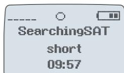
As the search progresses, monitor the screen until the signal bars indicate good signal strength (at least two bars), and the full circle symbol displays ●.
