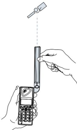
To do this, angle the phone antenna in the direction of the satellite.
