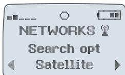
2. Using the left and right arrow keys, scroll to **NETWORKS/Search opt Satellite** and press **YES**.
