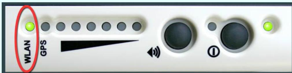
If WEP encryption is disabled, the WLAN LED lights red.
