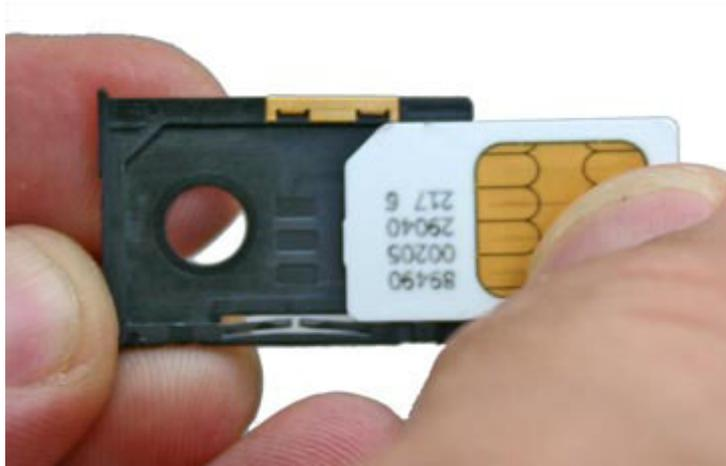
6. With the card in the holder, orient the holder with the card's gold contacts facing down. Place the holder back in its slot in the BGAN terminal.
