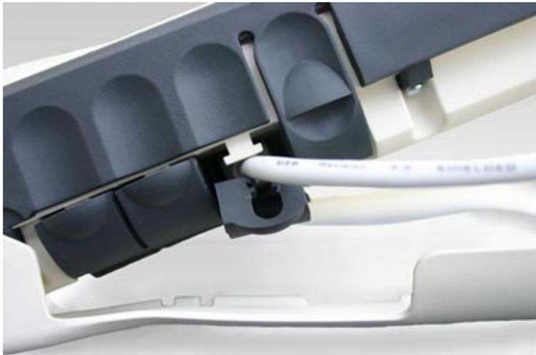
2. At the terminal connection point, slide the cable through the rubber door slot in order to secure and protect the connection.
