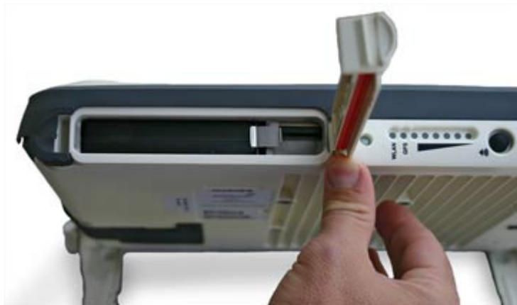
3. Push the button on the left-hand side of the SIM card holder. This releases the holder from its compartment.
