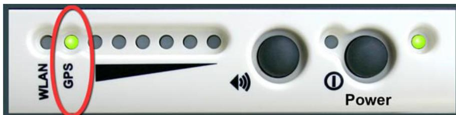
Leave the terminal to acquire a GPS fix. This may take a few minutes. Once the GPS fix has been acquired the GPS LED turns solid green.
