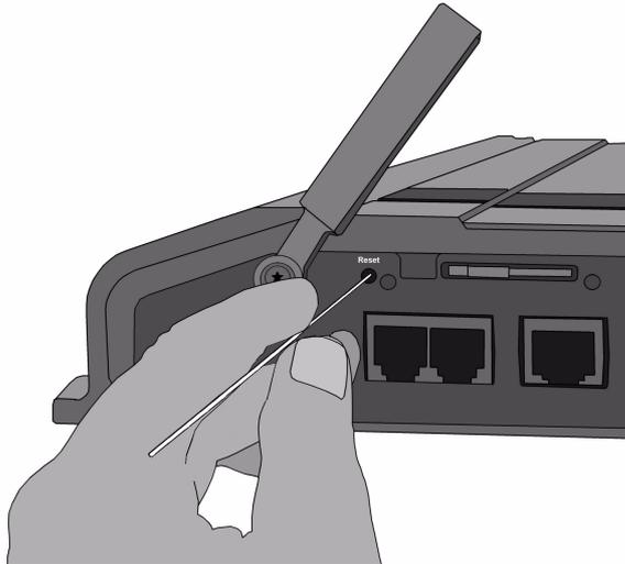
To press the Reset button, use a pointed device.
