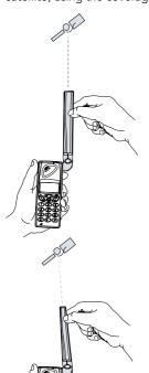
To do this, angle the phone antenna in the direction of the satellite.
